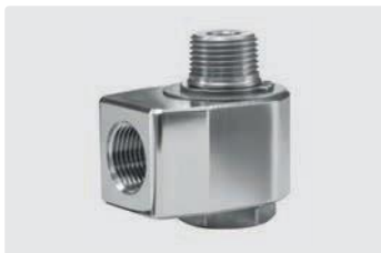
3/8" GW : 3/8" GZ. DN 7. Max. 275 bar / 30 r.p.m. / 120 °C
