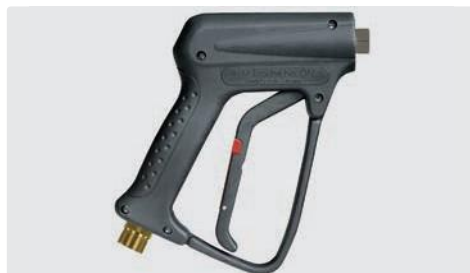
Pistolet R+M EcoLine No. ONE. Max. 250 bar / 45 l/min / 150 °C
