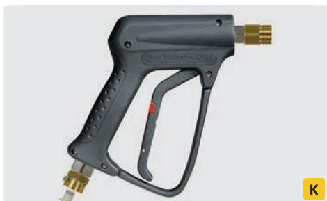
Pistolet R+M EcoLine No. ONE. Max. 250 bar / 45 l/min / 150 °C
