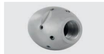
3/4" GW. 6x 75° 3x 30° +1x 0°. 100-250 l/min. Do \text{R} \text{D} 150-300 mm. Zewn. \text{D} 50 mm. \text{g} 1,367 g.
