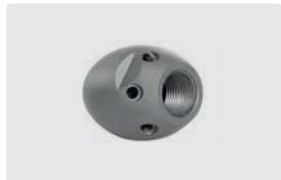
1/4" GW. 6x 75° +1x 0°. 20-50 l/min. Do \text{R} \text{D} 50-100 mm. Zewn. \text{D} 30 mm. \text{g} 127 g.
