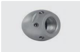
3/8" GW. 6x 75° +1x 0°. 25-70 l/min. Do \text{R} \text{D} 75-150 mm. Zewn. \text{D} 35 mm. \text{g} 207 g.
