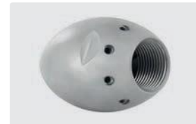
1" GW. 8x 75° +1x 0°. 100-250 l/min. Do \text{R} \text{D} 150-300 mm. Zewn. \text{D} 62 mm. \text{g} 1,265 g.
