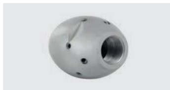
1/2" GW. 6x 75° 3x 30° +1x 0°. 80-140 l/min. Do \text{R} \text{D} 120-250 mm. Zewn. \text{D} 40 mm. \text{g} 630 g.
