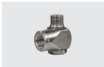
3/8" GW : 3/8" GZ. DN 6. Max. 400 bar / 30 r.p.m. / 90 °C
