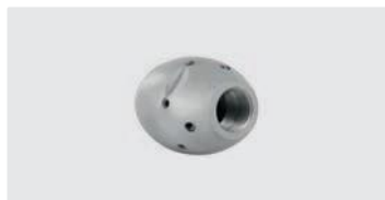
1/4" GW. 6x 75° 3x 30° +1x 0°. 25-70 l/min. Do \text{R} \text{D} 75-150 mm. Zewn. \text{D} 30 mm. \text{g} 223 g.
