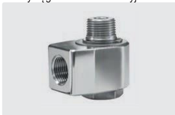
3/8" GW : 3/8" GZ. DN 7. Max. 275 bar / 30 r.p.m. / 120 °C
