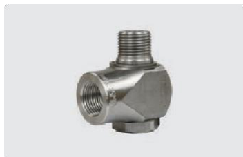
3/8" GW : 3/8" GZ. Max. 400 bar / 30 r.p.m. / 90 °C
